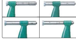
adjust collars for different measuring ranges
