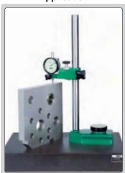
Rigid construction, designed to make comparison height measurement (set zero with gage block then measure height of workpiece) with dial indicators or digital indicators (variation of measuring force is high)
