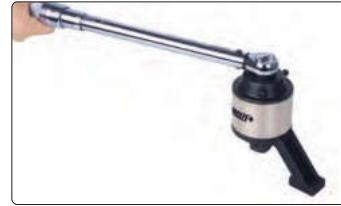
Example: the maximum output torque is 1000N.m (torque ratio is 1:4), the maximum input torque can not exceed 250N.m, otherwise may be damaged the torque multiplier
