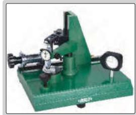
check the effect of lateral force on accuracy of test indicators
