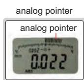
Read the diameter directly, after imputing the size of setting ring.
