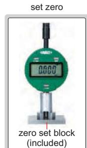
measure peak-to-valley height of blast cleaned surfaces
