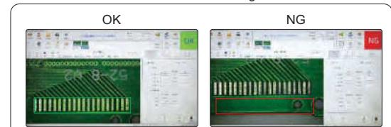
select the area and specify the target, the camera will automatically calculate the number of targets.
